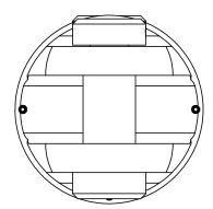
NOTES: -LOAD CAPACITY: 26 PIN MAX CAPACITY AT 9,000 LBS PER PIN (234,000LB BREAKAWAY MAX) -PINS SHOUD BE INSPECTED REGULARLY FOR CORROSION, PITTING OR DEFORMATION/DAMAGE AND SHOULD BE REPLACED IF ANY ISSUES FOUND -IDEALLY FOR CRITICAL APPLICATION WE DO RECOMMEND THE BE REPLACED FOR EACH USE
