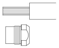
2. Slip the threaded cone nut over the exposed conductors.
