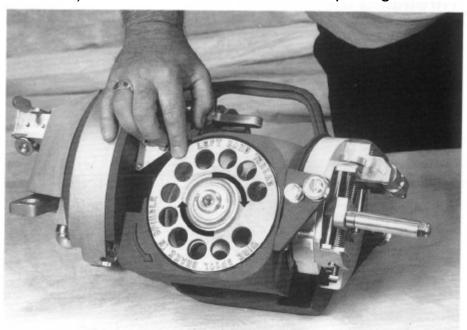
1b) Cut two wire ties. Insert coil of wire on spool so coil of wire will turn in a counterclockwise rotation (Right to left) when pulling on wire. (Load both sides to rotate in a conterclockwise direction). Cut and remove remaining twowire ties. Replace flange and tighten flange as tight as possible to keep coil of wire from turning on wire spool. (To hold wire spool from turning when tightening flange, insert finer in the hole located on back side of wire spool well at bottom.)
