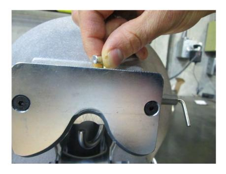
**4c)** When the lever is in the open position, pull it upwards to lock into place. The lever on the side of the strand lock should pop back in to lock the strand lock into place. Pulling the side lever out will once again unlock the strand lock.
