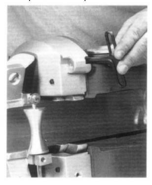
You are now ready to proceed to place the Lineman Lasher on the supporting strand. Position the cable in the lasher. Close front and rear gates. Adjust rear rollers to center cable. Raise the clutch handle to allow additional wire to be pulled out of the machine without rotating the machine to tie off lashing wire to strand. Attach towing rope to pulling rings on front of lasher.
