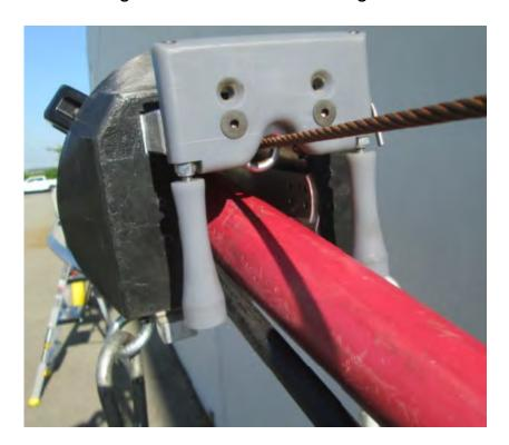
**8a)** To install, remove the bumper plate provided with your lasher by removing the two flat head screws on the front of the unit. Install the Overlash assembly in place of the bumper plate as shown so that the side rollers are in a vertical position at the front opening of the machine.
