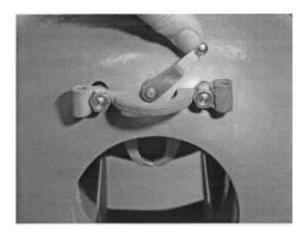
f. Place cable inside machine and close front cable placing rollers by pushing in on each until it snaps into place supporting the cable.
