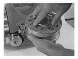
d. Tighten knurled knob by turning to the right.. Make sure wire spool is all the way down on the spindle before tightening.
