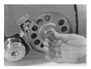
b. Remove the wire spool flange by turning clockwise.
