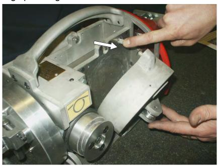
при Remove two coil ties from the wire coil and pull out approximately 12" of wire from inside of coil. Take loose end of wire and insert through wire guide in center of the wire magazine door pulling out at least a 12" length.
