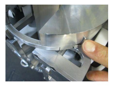
You are now ready to proceed to place the Eagle Lasher on the supporting strand. Position the cable in the lasher. Close front and rear gates. Adjust rear rollers to center cable. Raise the clutch handle to allow additional wire to be pulled out of the machine without rotating the machine to tie off lashing wire to strand. Attach towing rope to pulling rings on front of lasher.
