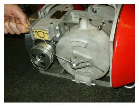
**2e)** When using non-metallic wire, it is recommended that the wire is threaded under the guide wheel on the lashing wire door as shown. This will ensure alignment of the wire to prevent it from falling off the drive wheel.
