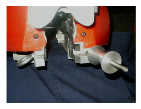
**3c)** To release drum lock, push front cable roller back to the closed position.
