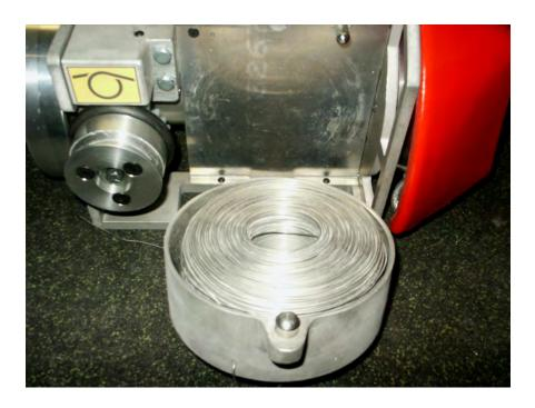
**1d)** It is optional to take the Outside coil of wire and, pulling out approx 12", feed it through the small hole in the outside of the magazine. This can later be attached to the body of the Lasher once the magazine is closed. This will prevent any possibility of the Wire coil spinning inside the magazine.
