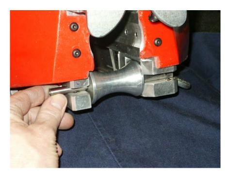
**3b)** Once the lock is released, swing roller completely open to clear the cable. This will engage the drum lock and keep the drum from rotating.
