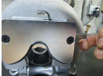
**4b)** Rotate the top lever back (approx. 270°) and pull up into slot to swing the strand lock out of the way. Note that the bend on the top lever matches the alignment of the strand lock, so the position of the strand lock can be known without having to look inside the machine.
