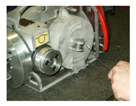
**2d)** Pass the wire over the guide roller on the magazine cover and then form a loop with the wire such that the entry onto the drive wheel is at the TOP and toward the outside of the drive wheel and the exit from drive wheel also at the TOP but toward the inside.
