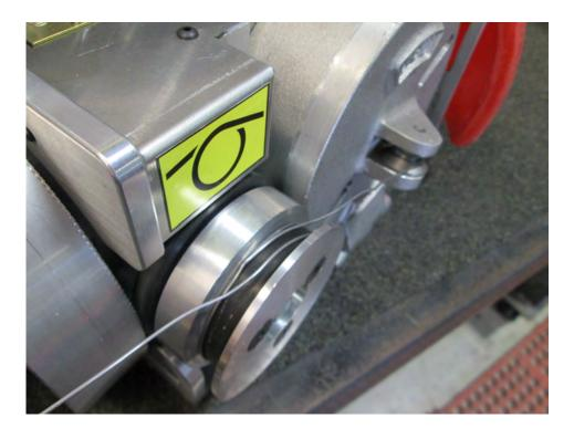
Note that the rubber tires may also be removed to reduce friction and pulling force, depending on your specific operating conditions.
