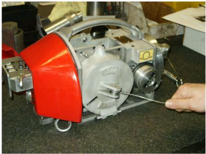
**2b)** Pass the wire over the guide roller on the magazine cover and then form a loop with wire such that the entry onto the drive wheel is at the BOTTOM and toward the outside of the drive wheel and the exit from drive wheel also at the BOTTOM but toward the inside.
