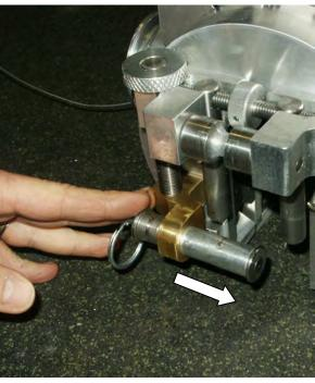
**5c)** To adjust the height of the rear gate roller up or down, scroll the knurled roller and the gate will wind up or down. During operation this gate should be set to within 1/8" of the cable.
