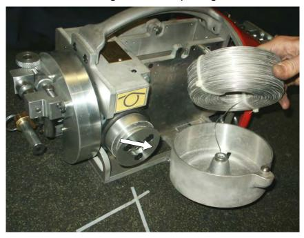
**1c)** Place coil in magazine. Remove the last two wire ties and close magazine door. Load the second wire magazine in same manner.
