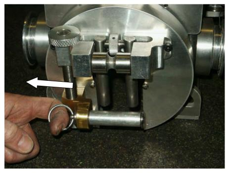
**5b)** To close rear gate, simply push gate roller back in and it will click into the closed position.
