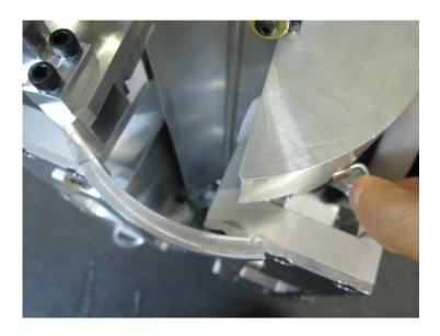
**5b)** When closing, the rear cover can be pushed and snapped back into the closed position. Pull the lever on the right to allow rear cover to swing open. Open it fully by hand to lock it in the open position. Ensure that the lever is tucked against the side of the lasher to prevent interference during rotation.
